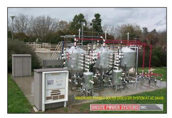
**Second phase pilot digester development** started in 2002 when OPS dismantled the 1,800-gallon Pilot plant and constructed a larger 14,000-gallon total reactor volume pilot APS digester plant at the site of the new UC Davis wastewater plant. The primary function of the second phase pilot system was the evaluation of a variety of commercially available equipment and components.
