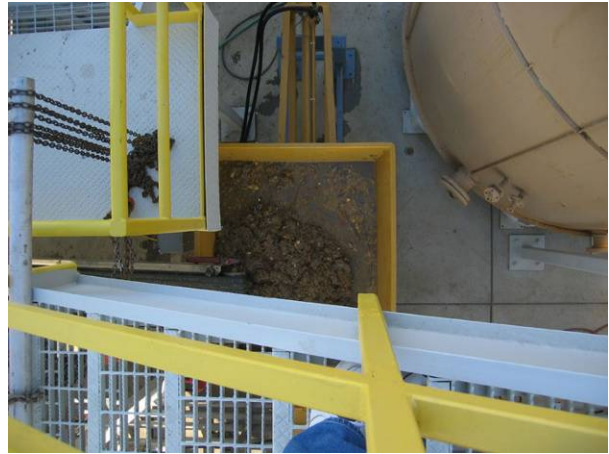
6) This view is of the hopper holding a load of food waste.
