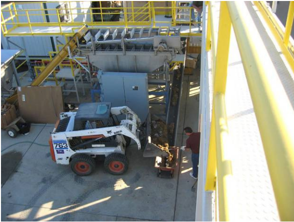
5) The waste is loaded onto a conveyor which quickly carries it up to the hydraulic ram pump hopper.
