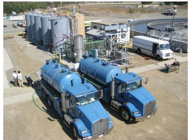
8) On October 13, 2006, two 3,500-gallon trucks bring 6,000 gallons of anaerobic, thermophilic digester sludge from East Bay Municipal District to Onsite Power Systems' APS digester plant at UC Davis. The sludge contains the methane-producing bacteria to populate the methane generating gasification tank.
